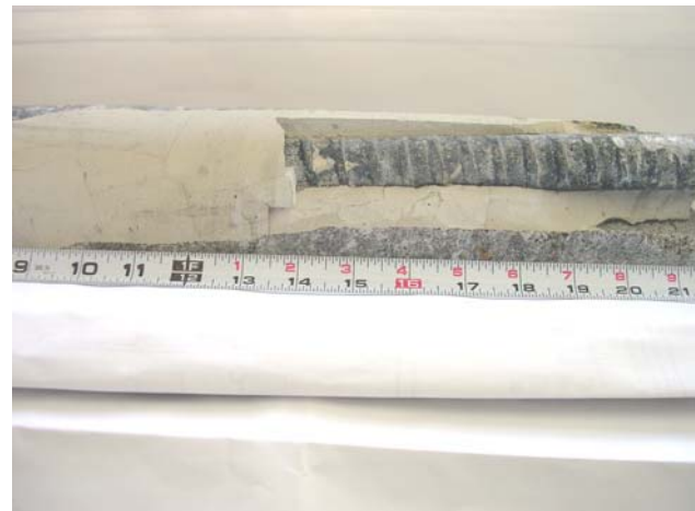
FIGURE 6. Tendon Element 2-4 With Portland Cement Grout Retrieved Near Proximal End.
